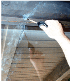
smokestick infiltration test Photos: House Energy Doctor
